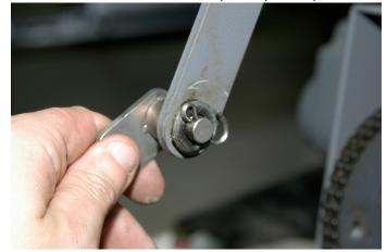
Install a washer and cotter pin thought the hole in the post. Bend cotter pins around completely so they do not snag or catch against anything.
