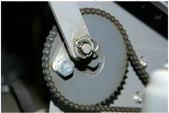
Holding the trap machine up, position the pivot arm toward the top of the gear and hand tighten the bolt through the threaded hole in the gear. The wobble limiter may rest against the center shaft of the gear to make it easier to tighten the bolt.
