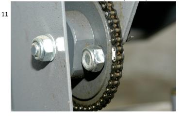
Install the nylon lock nut on the bolt to the left side of the gear. Lighten tighten with a wrench until the nut just touches the gear.
