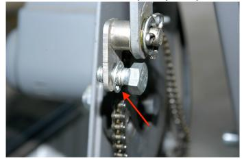
Insert a 1 ½ 10 mm bolt with a star type lock washer through the hole on the wobble limiter. The washer provides a "grip" surface to prevent the part from slipping when installed. Arrow shows the location of the lock washer.
