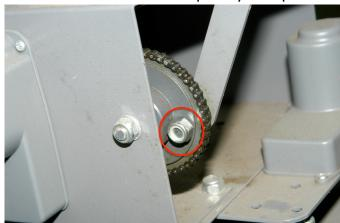
Using a 17mm open end wrench, remove the nylon lock nut located to the left of gear drive.
