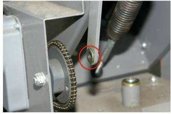
Once the bolt has been removed, make sure the brass bushing is still in place on the pivot
