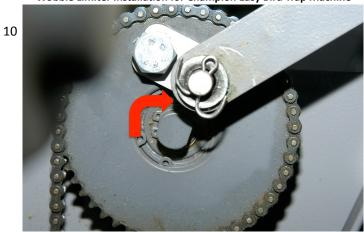
Place a flat washer between the wobble limiter and the center post to serve as a spacer. This will create about 1/8" of clearance to prevent the limiter from rubbing or binding when being used. The arrow in the picture indicates where the washer should be placed. Using a wrench, tighten the bolt firmly to the gear. Do not over tighten to prevent damage to the gear.
