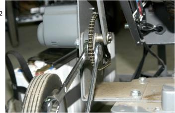
Place a wrench on the bolt head attaching the wobble limited to the gear and using a second wrench, snug the nylon lock to prevent the limiter from slipping. The wrench on the the bolt head should be used to prevent the limiter from shifting when tightening the nuts. Once tighten, you can use a pair of pliers to remove the washer that was serving as a spacer between the limiter and the near shaff
