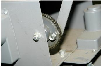
Power wobble attachment unit on and allow the wobble gear to rotate forward so the bolt assembly attaching the arm is in the forward most position. Make sure the main unit is powered off and the throwing arm is not cocked. Disconnect all components from the power supply before continuing.
