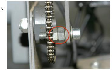
Using two open end wrenchs, loosen bolt from the gear slightly and separate the two nuts that are jammed together so they turn freely. Holding the nuts, back bolt out of gear.
