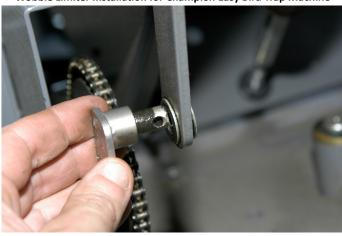
Insert the limiter through the pivot arm on the left. There is no need to use a washer since the shoulder of the post and the bushing in the pivot arm serve this purpose.
