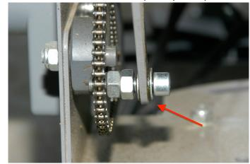
When removing the bolt, the two nuts that served as spacers should stay close to the gear to keep the pivot arm from binding. If the nuts move with the bolt, the pivot arm will bind and the bolt can not be completely removed or the threads in the gear could be damaged.
