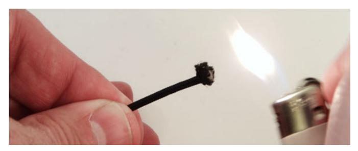
A properly melted end will not have any charring, ash, bubbles or anything else that will weaken it. If you have any of these defects, throw the loop away and start again. It is not worth the risk of having an improperly melted loop pull free or break.
