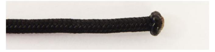
Repeat for the other end and measure the final product. You should have between 4 and 4 1/2 inches BETWEEN the finished melted ends.
