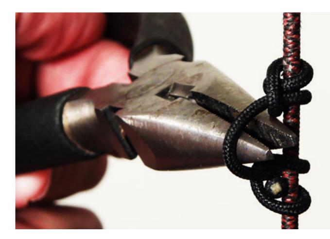
If you are still tuning your bow and are not sure of exactly where arrow nock should be located, leave the knot a little loose so that it can be moved up and down the bow string. Moving it can be done by screwing it up or down as it will follow the winds of the bow string serving.
