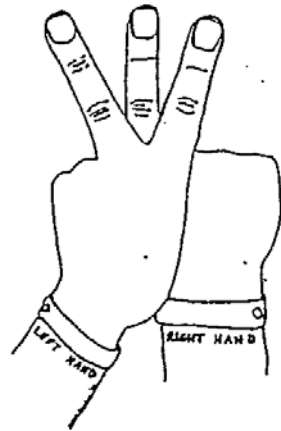
Figure A-1: Two fingers of left hand simulate rear sight. Index finger of right hand simulates front sight. Represents perfect sight alignment.
