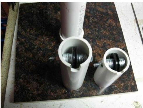
Cut a notch no more than ¼" wide and ½" in for the line to run through. This will be used to trap the fender washer and keep the pistol hook from being pulled into the pulley, derailing the line.
