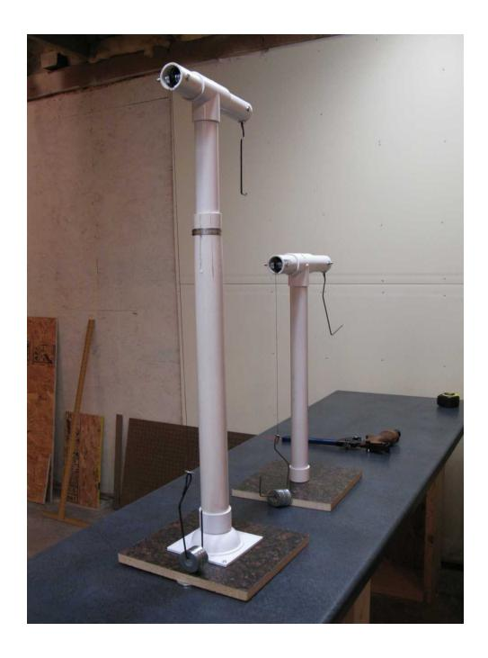
There you have it. Two very simple pistol slings that are inexpensive and easy to build. To adjust the amount of lift on the pistol simply add or remove washers to the counter balance. You will notice the weights swaying when held in suspension by the pistol. This movement can not be felt by the shooter. Feel free to modify, improve and customize these slings to suit your needs.
