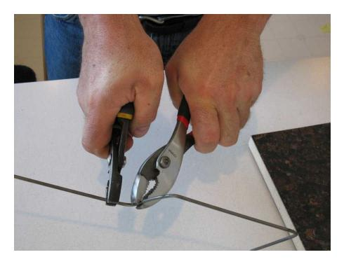
The sizes shown in the picture work well for us but are by no means mandatory. I recommend that you do not put an up turned "hook" on the horizontal bar that the pistol rests on. It serves no real purpose and snags the gun if the shooter does not lift the gun all the way up.
