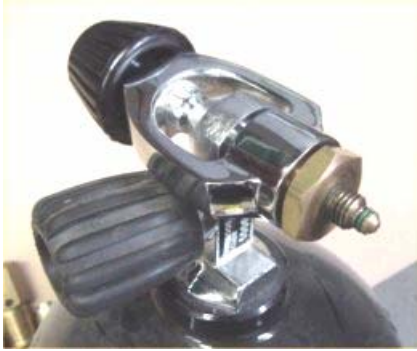
D-yoke and adapter installed on a SCUBA tank with a K-valve
